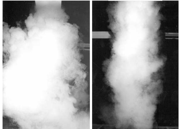
Figure 4: Jet dispersal made visible with a smoke tracer, left: cooling mode; right: heating mode.
